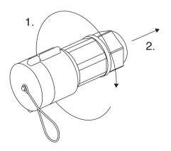
4 Fix the cable. This sign must be on top: < \_\_\_\_\_</p>
